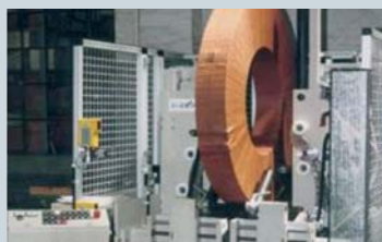
Vertical wrapping machines for crane or forklift truck loading. Semi- and fully automatic solutions.
