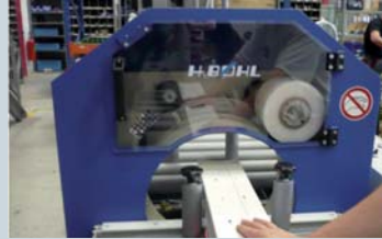
Semi automatic BSB-450 SX with 125 mm film width
